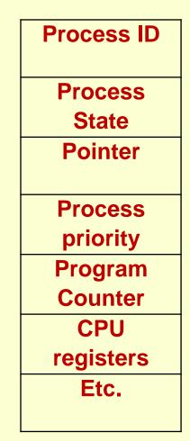
A typical Process Control Block
